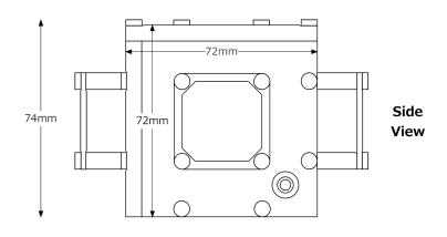
$72mm = 1\lambda \text{ of } 4700Hz = 0.5\lambda \text{ of } 2350Hz$
